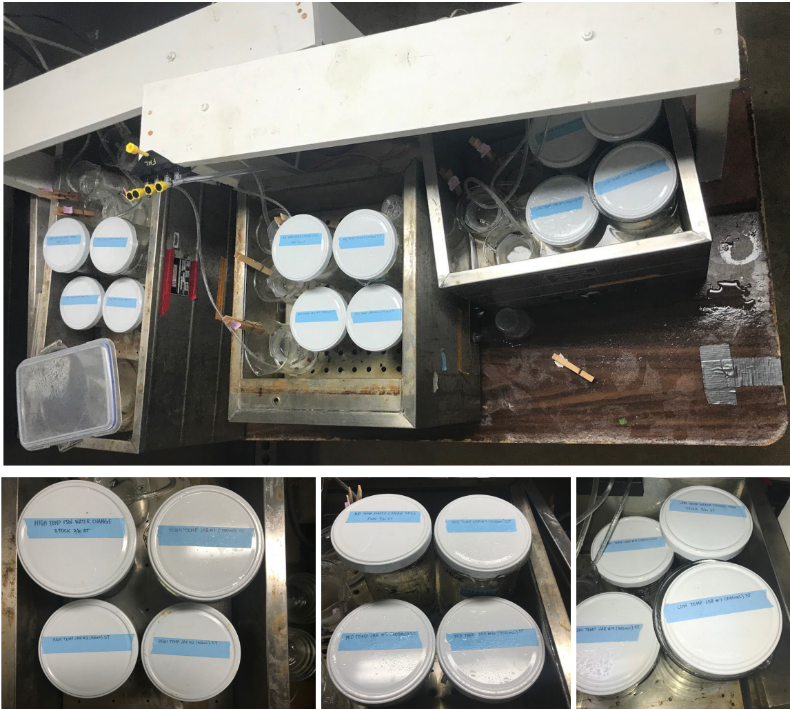
Figure 2. Experimental setup, involving three water bath apparatuses in a cold culture room kept at 10.5°C. The highest temperature water bath resides on the left, and lowest temperature (control) resides on the right. Images taken with an iPhone 7, on the first day of treatment.
