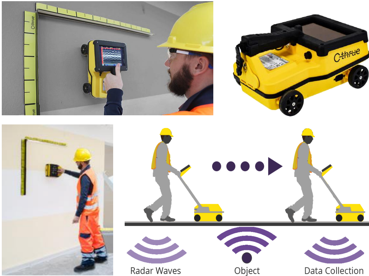
FIGURE 12 - UPPER LEFT IMAGE, CLOSE UP OF C-THRUE IN USE WITH WAVE FORM READOUT DISPLAY IN VIEW, BOTTOM LEFT, TYPICAL VERTICAL SURFACE SCAN, UPPER RIGHT, C-THRUE GPR SCANNER, RIGHT, DIAGRAM OF C-THRUE HORIZONTAL SURFACE SCAN OPERATION AND WAVE FORM FUNCTION. “C-THRUE.” IDSGEORADAR.COM, HEXAGON, IDS GEORADAR, 2024, IDSGEORADAR.COM/PRODUCTS/GROUND-PENETRATING-RADAR/C-THRUE.
