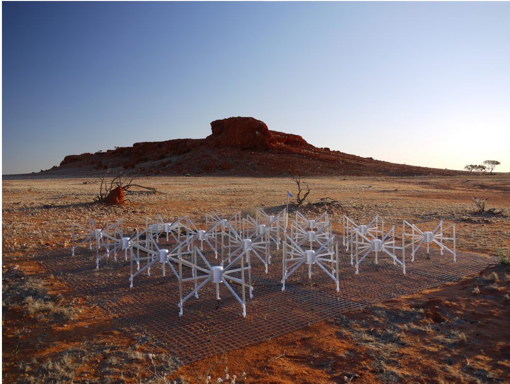
Figure 1.2: A 4x4 tile of crossed dipoles antennas that form a single receiving element of the Murchison Widefield Array, a radio interferometer located at the Murchison Radio Observatory in Western Australia. Radio interferometers cross-correlate electric field measurements from multiple receiving elements to form visibilities. These visibilities can then be used to construct images of the radio emission on the sky. Photo credit: Dr. Natasha Hurley-Walker.
