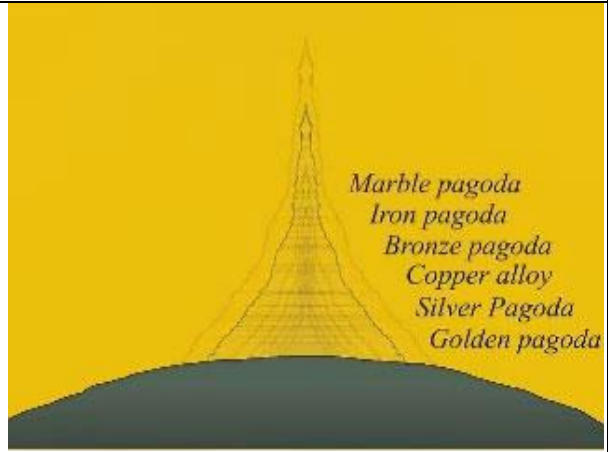
Figure 4.5 Schematic diagram of Shwedagon's 7 layers encased pagoda. (Ashin, 2008: 330)
