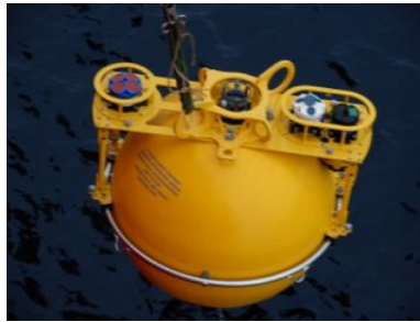
Figure 2: Mooring during deployment. The AWAC is on the right-hand side (white and blue sonar head).
