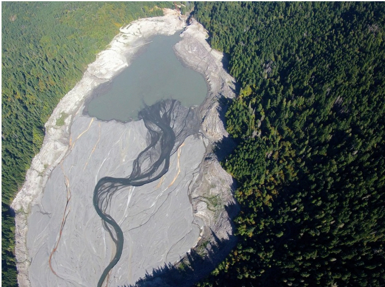
Figure 18: Lake Mills is drained following the removal of the Glines Canyon Dam (Source: Tom Roorda)
