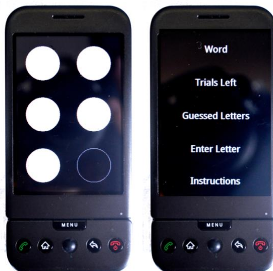
Figure 4.1. The VBraille interface for “reading” and “writing” Braille characters (left) and a menu from the VBHangman game that is based on the word game Hangman (right).
