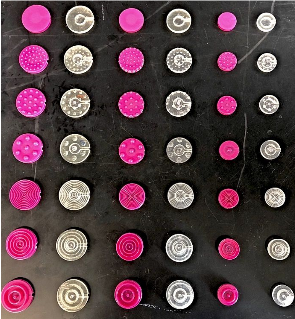
Figure 4.3. All 42 factor housings, arranged in rows by surface geometry and in columns by contact area. The clear housings are printed in compliant material, and the magenta housings are printed in stiff material.
