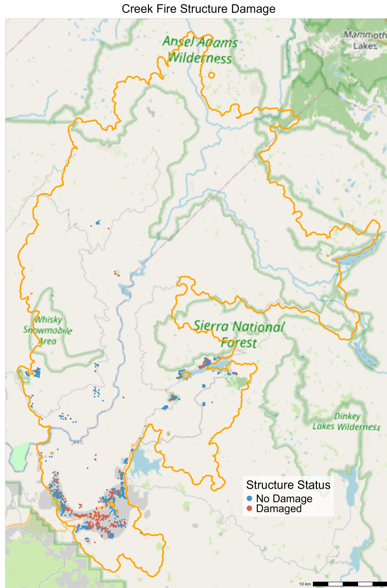
Figure 3.2: Locations of structures within the Creek Fire perimeter, classified by damage status from the CAL FIRE Damage Inspection (DIS) database. Points show structures that were destroyed ( >50\% damage, red) or undamaged (blue) following the 2020 Creek Fire in the southern Sierra Nevada, California. Most structures were concentrated in the southern portion of the fire near the communities of Pineridge and Shaver Lake.
