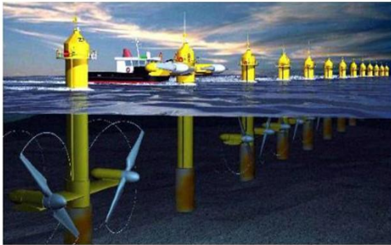
(b) Marine Current Turbine's SeaGen 1.2MW
