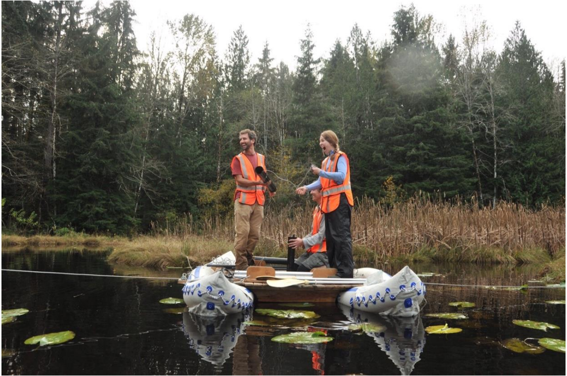
Figure 9. Coring raft on the Rowan Landslide pond. Pictured: Geoffrey Malick, Western Washington University, Dr. Doug Clark, and the author, Susan Wisehart. Geoffrey Malick is holding the core barrel, Dr. Clark is holding the casing in the core hole, and Susan Wisehart is holding the piston wire. Photo by Hannah Letinich.
