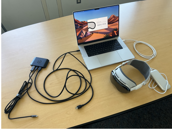
Figure 3.5: CARE platform wired latency testing setup.
