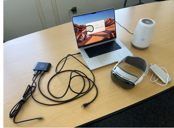
Figure 3.6: CARE platform wireless latency testing setup.
