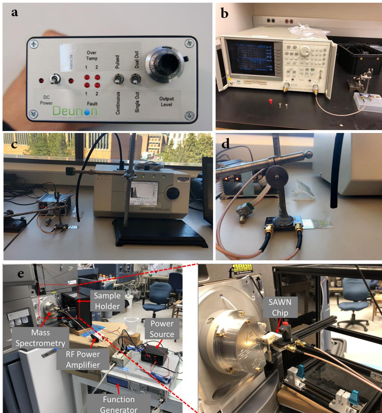
Figure 5.4. (a) Deurion SAWN power supply. (b) S parameter measurement setup. (c) Droplet size distribution measurement with aerodynamic particle sizer spectrometer. (d) Droplet nebulization and size distribution measurement.
