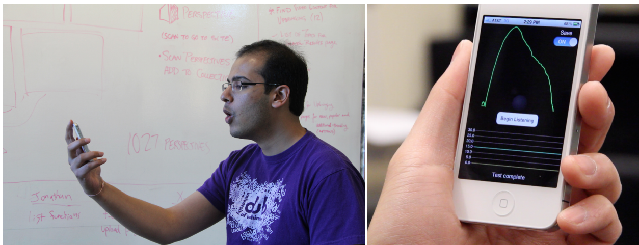
Figure 5.1: User using SpiroSmart. The maneuver on SpiroSmart is exactly the same as on a clinical device, except the lack of mouthpiece.
