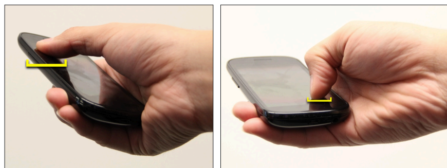
Figure 3.11: (left) Touch size is bigger when a far side is touched. (right) Touch size is smaller when a near side is touched.
