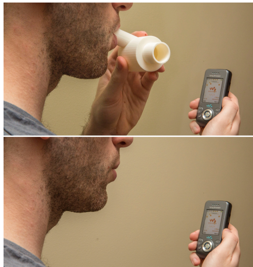
Figure 5.29: A user using SpiroCall on a feature phone (Sony w580i) with and without a vortex whistle.
