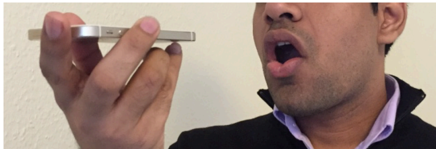
Figure 5.20: Participant using the application at a wrong angle. The app uses the gyroscope to check for such mistakes and notifies the user.
