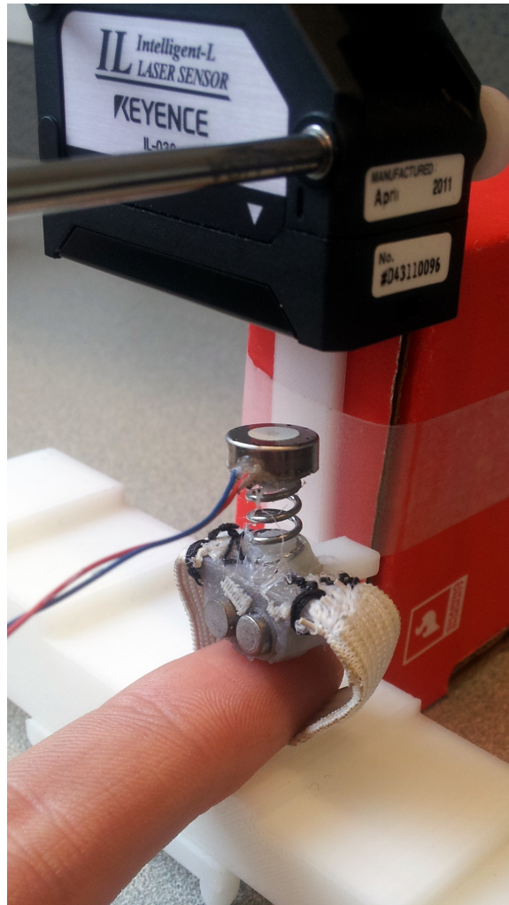
Figure 3.2: The prototype impedance adapter in test setup for displacement measurement.
