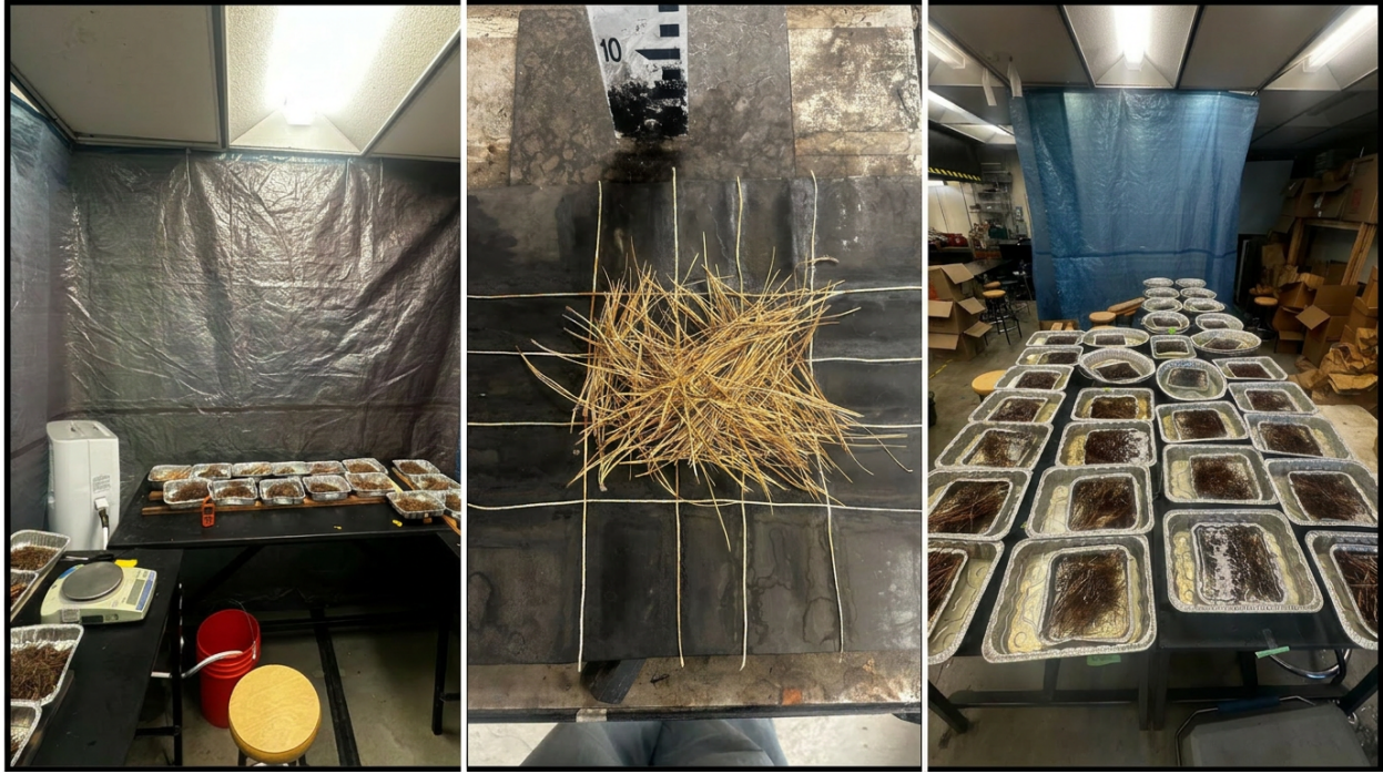
Figure 39. Laboratory experimental setup for fuel bed flammability trials conducted at California State Polytechnic University, Humboldt, August 2025. Left: fuel bed samples drying in the drying chamber. Center: a 15 g ponderosa pine fuel bed arranged across the wire grid before burning, with xylene-soaked strings used for ignition. Right: fuel bed samples fully submerged in water during the saturation phase. Photographs by Priscilla Sperandio.
