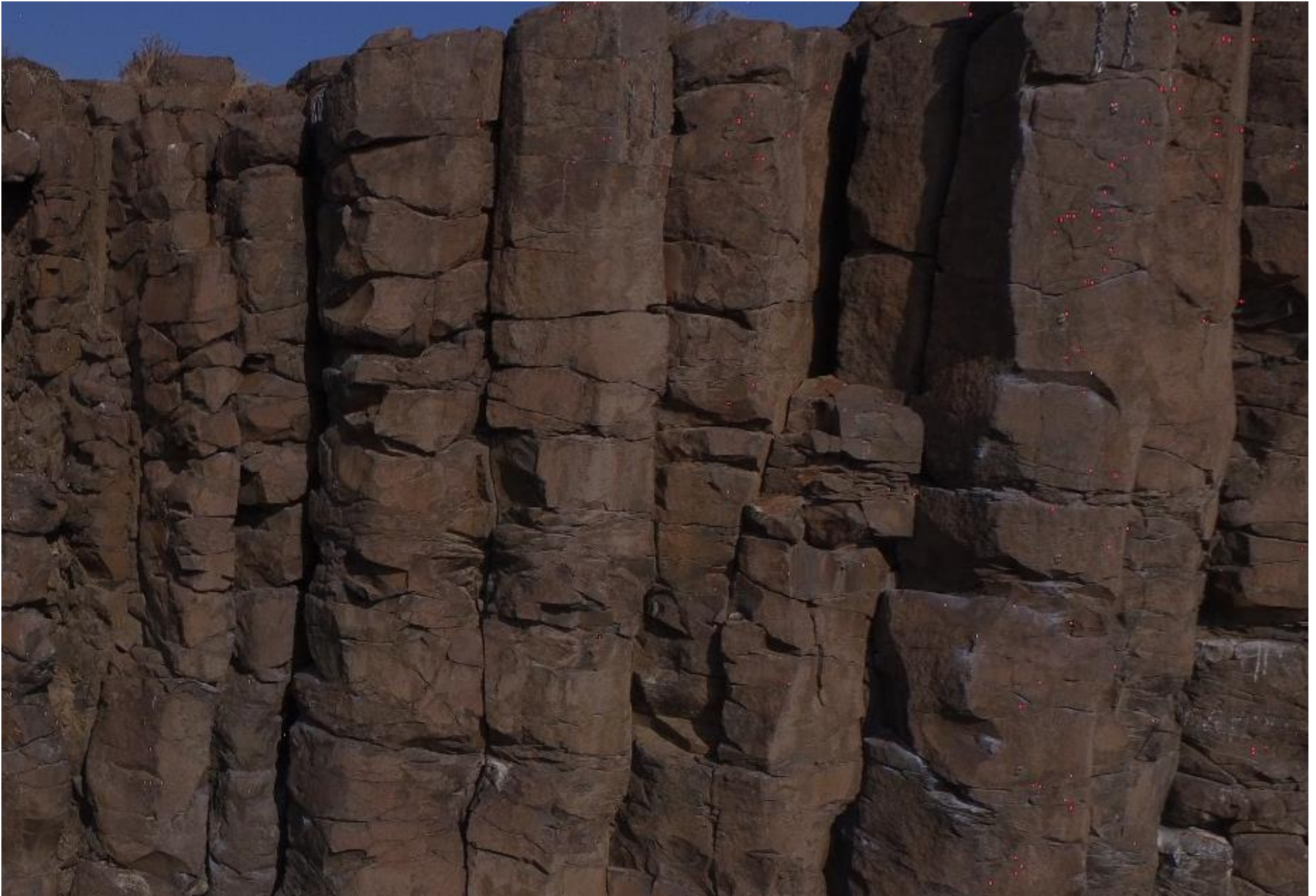
Figure 11b: This image shows a number of sub-horizontal fractures that are represented by poles plotting in the center of the stereonet. In the upper right corner of the image a set of chains are present, which are used by climbers to descend off the route.
