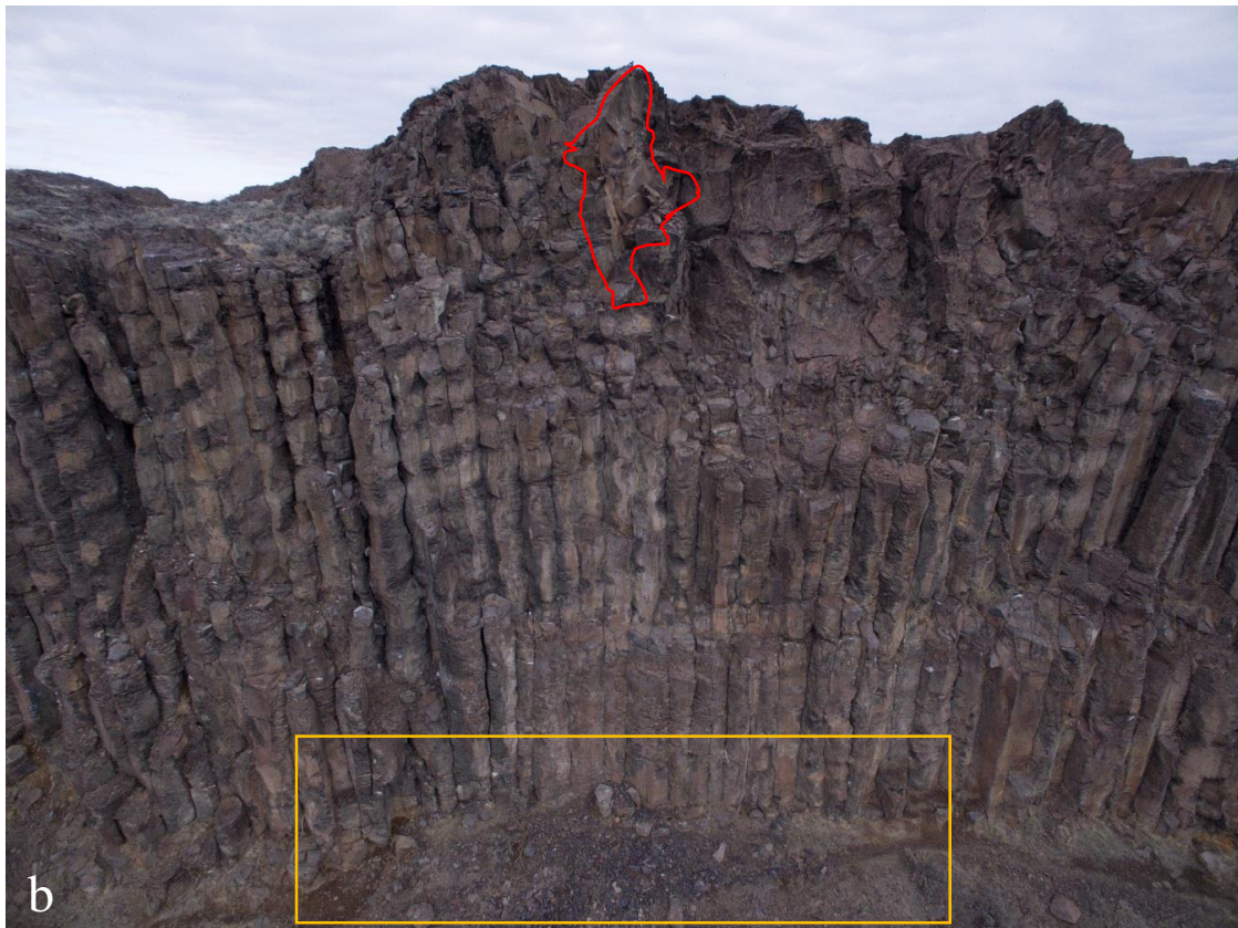
Figure 5: November 2018 Rockfall. These images show a specific section of the Sunshine Wall that was subject to rockfall in late November 2018. At the top of the page the specific block that detached from the rock slope is outlined in red. This picture was taken in October 2018 prior to the event. Below, is an image of the area after the rockfall event. Outlined in Red is the detachment zone. The block that fell was approximately 33 m 3 , which is the size of a Volkswagen Beetle. Shown below in yellow is the 33 meter section of trail that was covered in freshly broken talus. The rock is blueish in color due to the freshly fractured-unweathered surfaces.
