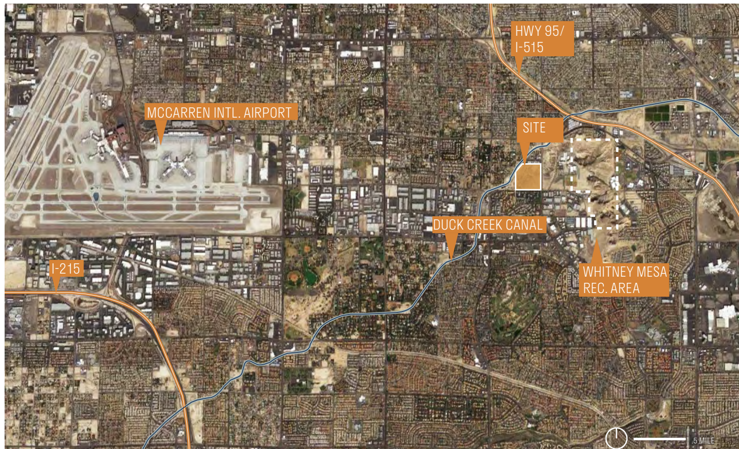
Figure 4.11 The Duck Creek Canal passes by the located site. This canal is one of the larger stormwater canal systems working to prevent flooding in the urban Las Vegas Valley. Image from Google Earth.
