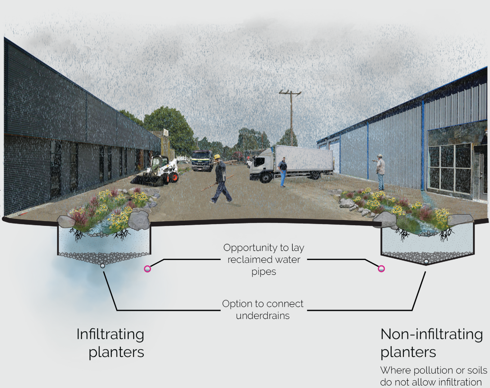
Figure 7.14: Section C. industrial swale islands with infiltrating (left) and noninfiltrating (right) examples
