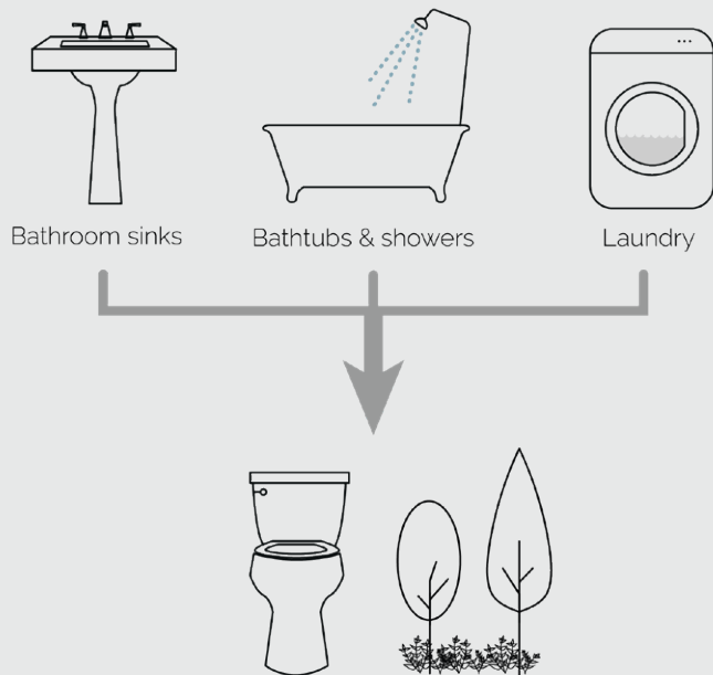
Figure 0.4: Types of graywater acceptable for reuse. Kitchen sink water is also considered graywater but contains more pathogens.
