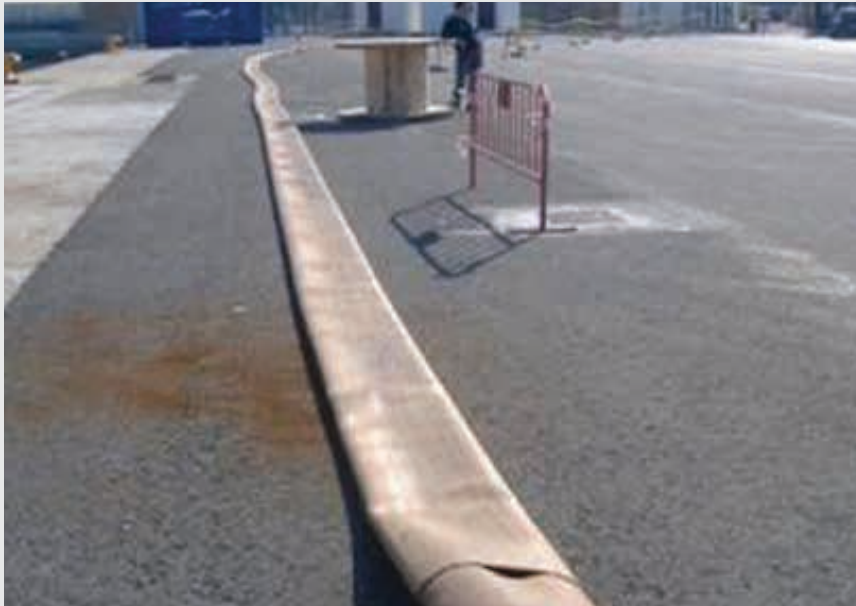
Figure 7.3: example of a how a lay flat hose can be manipulated to direct water (72)
