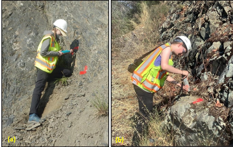
Figure 2.2 Acquisition of Schmidt hammer (SH) readings at sites in (a) Alaska and (b) Oregon.
