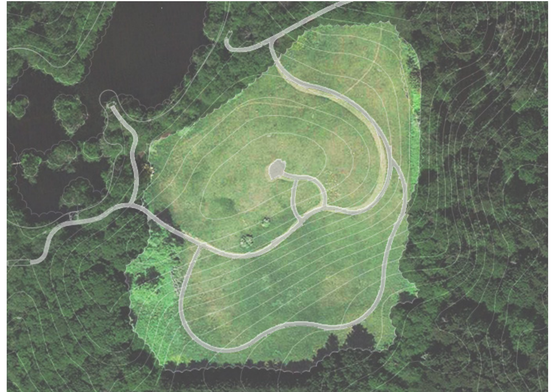
Figure 4.24: Contour lines overlaid on to a satellite image. Image Credit: Author
