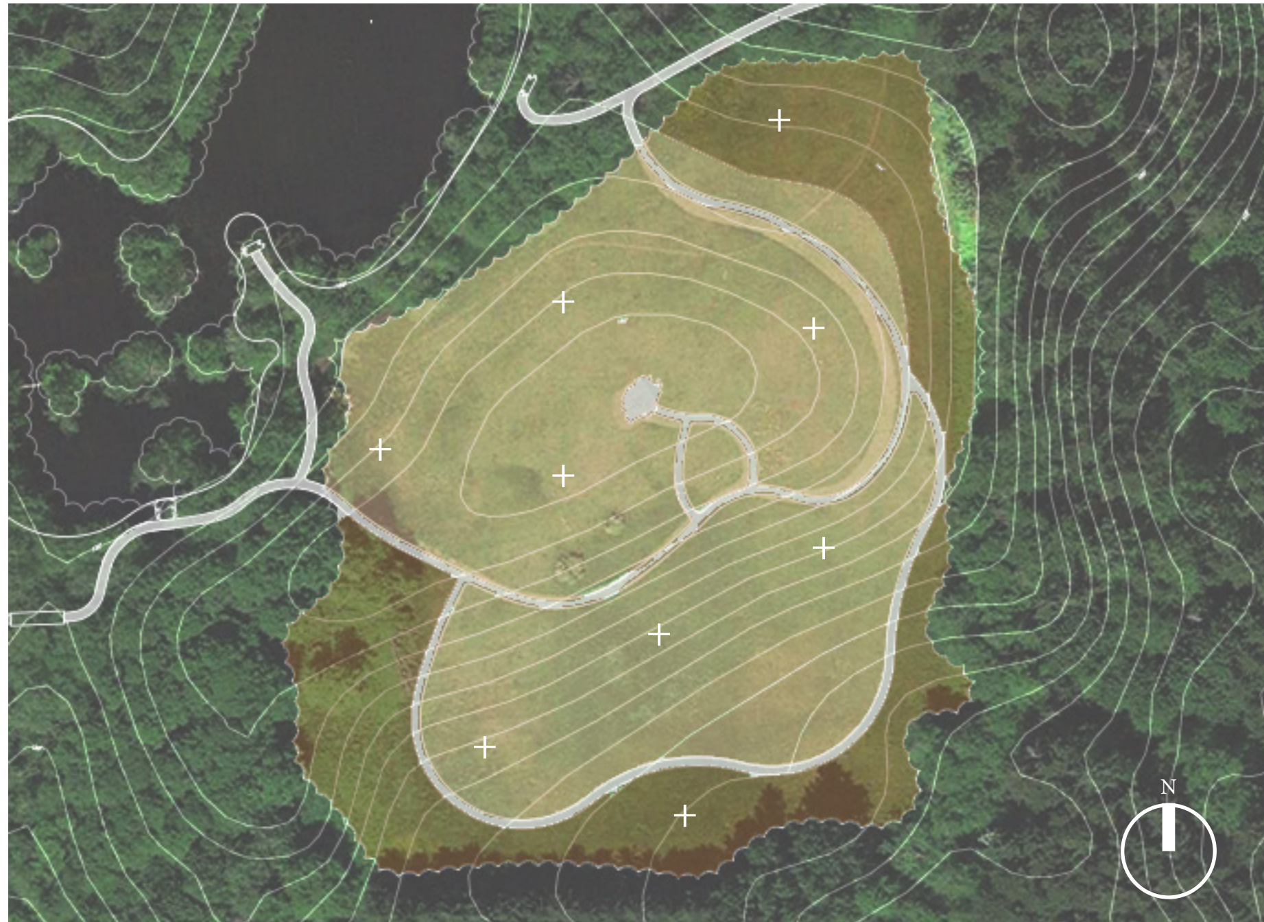
Figure 4.47: Plan view graphic showing two different soil types, and locations of soil samples. Image Credit: Author
