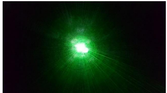
Figure 29: 532nm notch filter glare production at 60°
