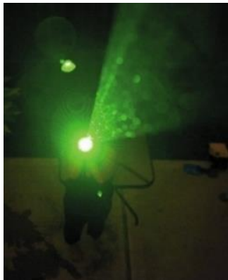
Figure 1: a demonstration by the USCG to show just how disruptive to the visibility and night vision of pilots laser pointers can be (Negroni 2013).
