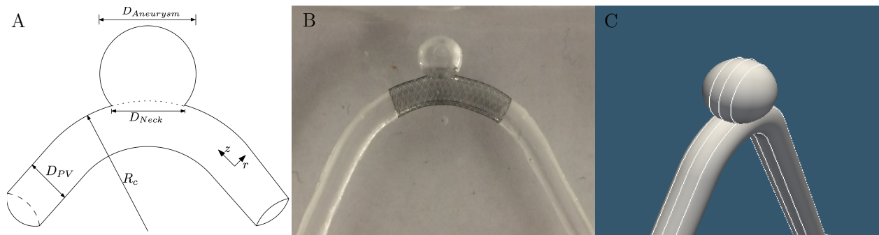
Figure 4.1: (a) Sketch of the idealized cerebral aneurysm with the key geometrical parameters used to define the study. (b) Silicone model of a side-wall cerebral aneurysm treated with a clinically-used stent along the parent vessel. The curvature in this case is 0.03\text{mm}^{-1} and (c) locations of the three laser planes used to image flow in the aneurysm models.
