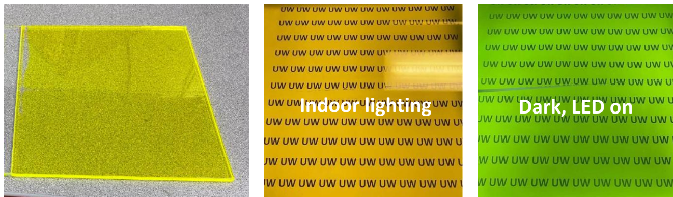
Figure 3.14. (left) as-fabricated waveguide by blade-coating the Theo-Green-SBS composite on a glass substrate; (middle & right) demonstration of transparency and non-glare feature of the edge-lit lighting device based on the waveguide shown on the left.
