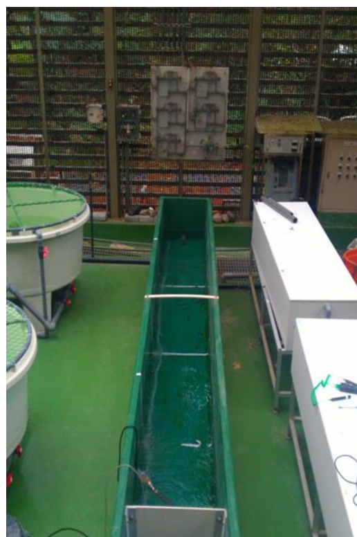
Figure 2.2. Photo of the experimental temperature gradient flume used to determine the temperature threshold at which salmon would express temperature avoidance behavior. This experiment was set up in the Taiwan salmon hatchery adjacent to the research site.
