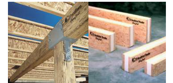
FIGURE 3: Laminated Strand Lumber is similar in composition to OSB, but with layers oriented parallel with one another. Commonly it is used for beams and headers, but the large billets in which it is manufactured are suitable for large panelized structural systems as well. (Images from Weyerhaeuser)
