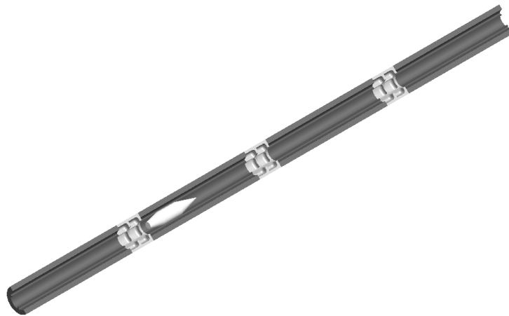
Fig. 2.11 Schematic of the RTRA with sweeper baffles.
