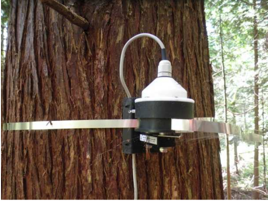
Figure 8. Dendrometer module, showing stainless steel band and rotary position sensor. The band is placed under tension during installation and changes in rotary position are recorded with 1 \mu\text{m} precision.
