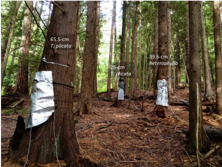
Figure 5. A photograph of the project site showing trees instrumented with sap flow meters and dendrometer bands. Camera is facing upslope and approximately north.
