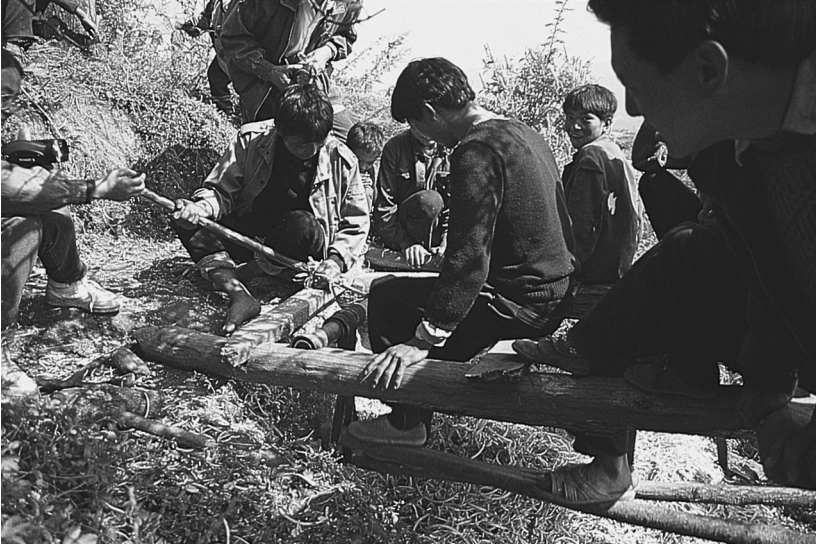
FIG. 6. Turning a bowl on the pit-lathe
