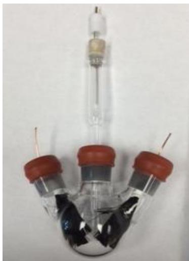
Figure 1.4. ROMP via bulk electrolysis (set-up).
