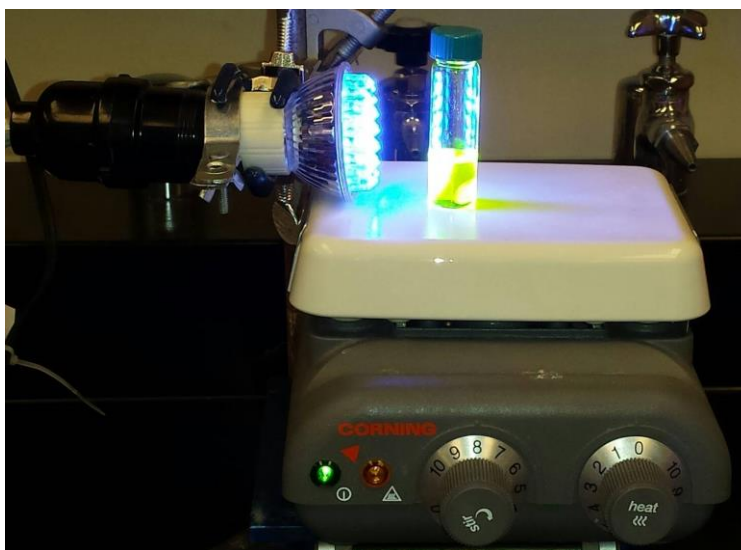
Figure 2.13. Polymerization setup for MF-ROMP of NB. The reaction mixture was stirred and irradiated for 75 min at a distance of 1 cm using a 2-W (total output) blue LED light source.
