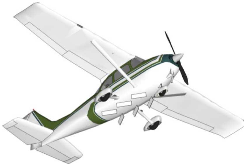
Figure 2.2: Concept drawing of antenna installation under the belly of a Cessna 172 aircraft.
