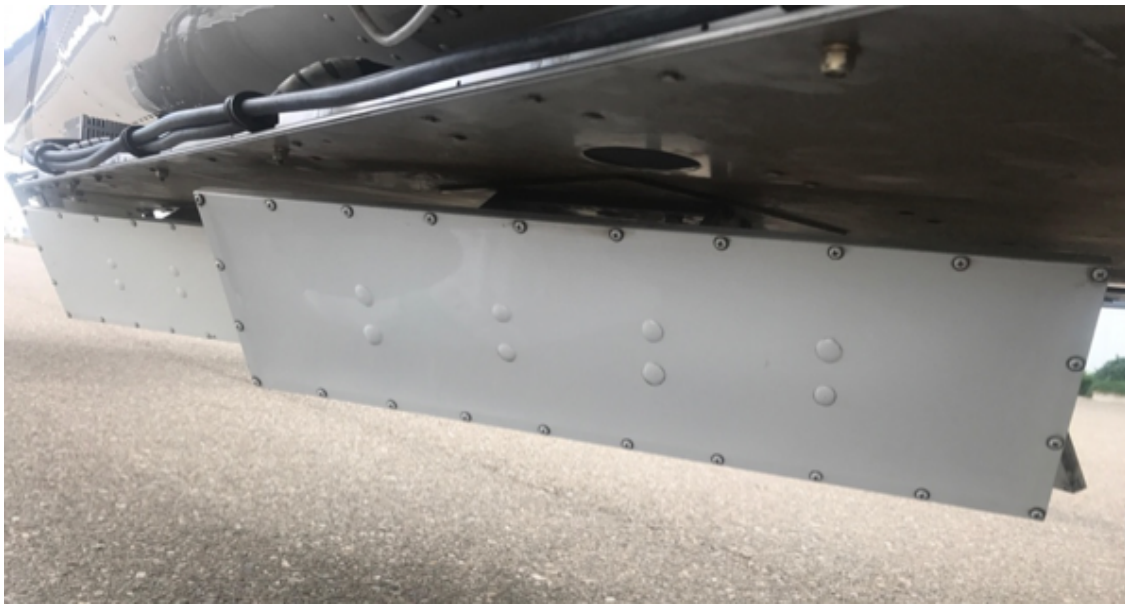
Figure 4.2: Picture of C-band patch array antenna mounted on the belly of the aircraft.
