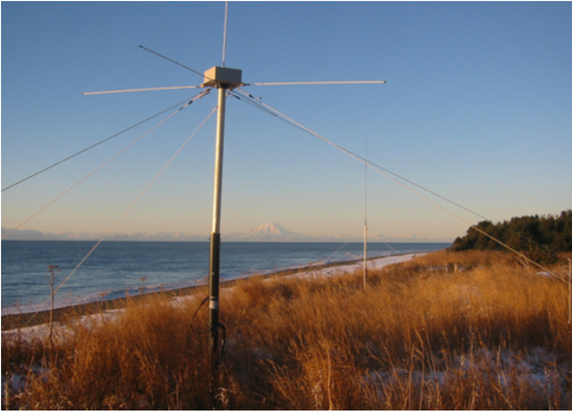
Figure 1.2: Near-shore high frequency radar developed by Qualitas Environmental Solutions for the measurement of surface currents and waves with a measuring range of up to 200 km. Reprinted from [2].
