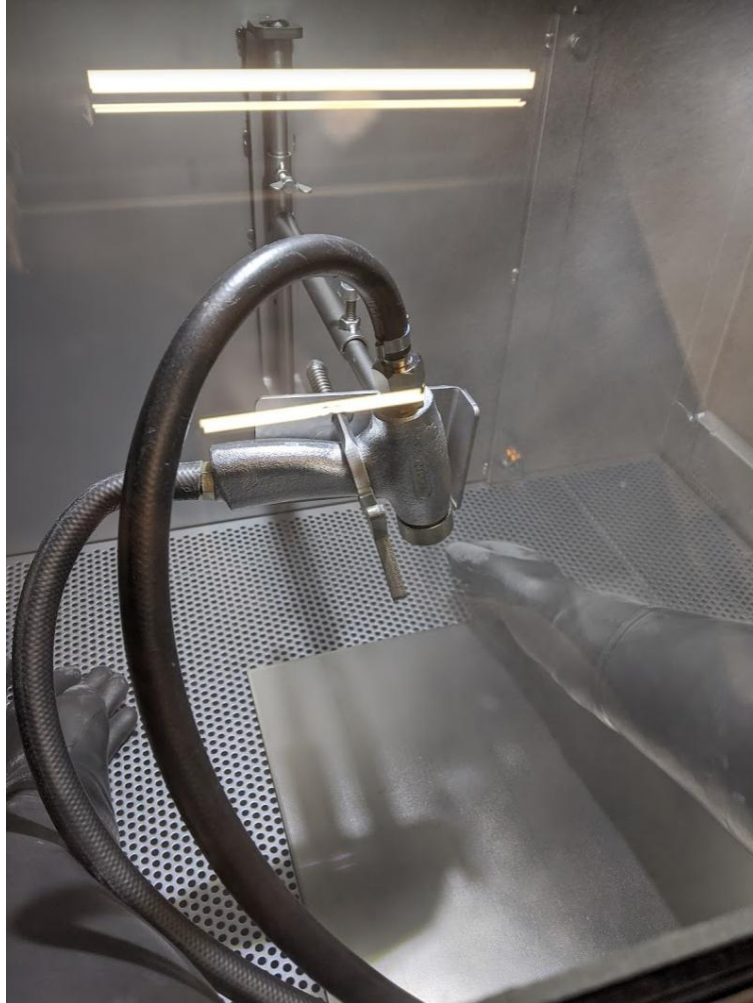
Figure 14: PRS chamber in which produced specimens were air blasted
