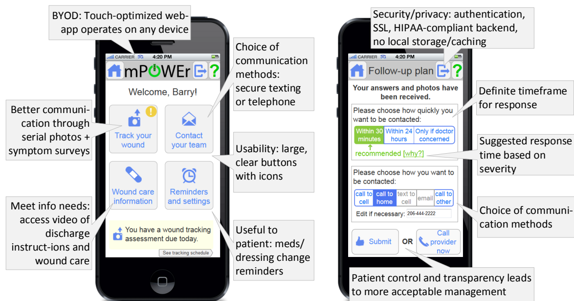
Figure 4-3. Application of design considerations to a wound tracking app. Each callout represents one of the 11 guiding themes that emerged from interviews with patients who experienced post-discharge complications.
