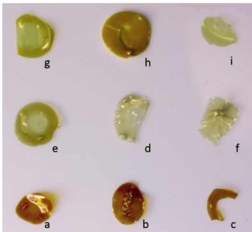
Figure 17. Nine polyimide films: a) PMDA-ODA, b) PMDA-PDODA, c) PMDA-FNDA, d) 6FDA-ODA, e) 6FDA-PDODA, f) 6FDA-FNDA, g) BPDA-ODA, h) BPDA-PDODA, i) BPDA-FNDA.
