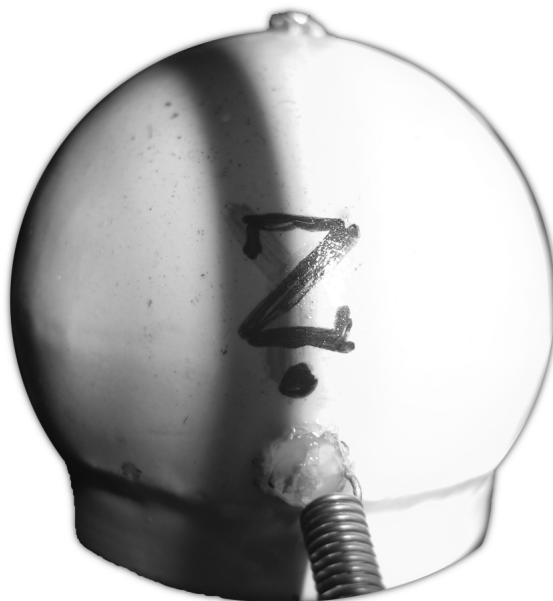
Figure 5.3: Neutrally Buoyant Housing of MOD-1 .
