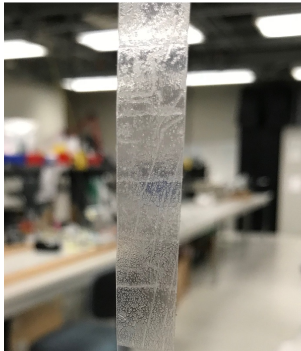
Figure 3.20. UnTape Medium Tack Tape Residue After Acrylic Test
