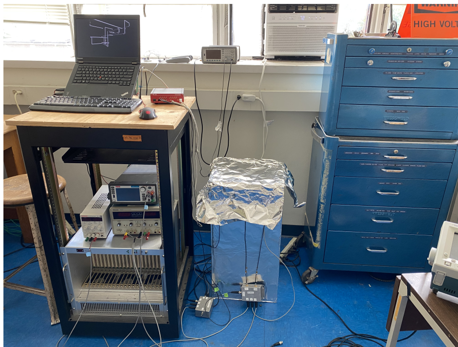
Figure 5.9: The SiPM characterization test stand. The dewar with the integrating sphere inside is located inside of the dark box which is covered on the outside with aluminum foil. Outside of the dark box are the second stage amplifications of the SiPM and APD and are read out by a CAEN DT5730 digitizer.
