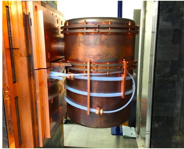
Figure 2.8: One of the detector modules outside of the shielding. The ^{228}\text{Th} source is inserted into and retracted from a plastic tube that wraps around the module. Fig. from ref. [70].
