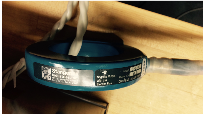
Figure 3.9: Stangenes Current Transformer
