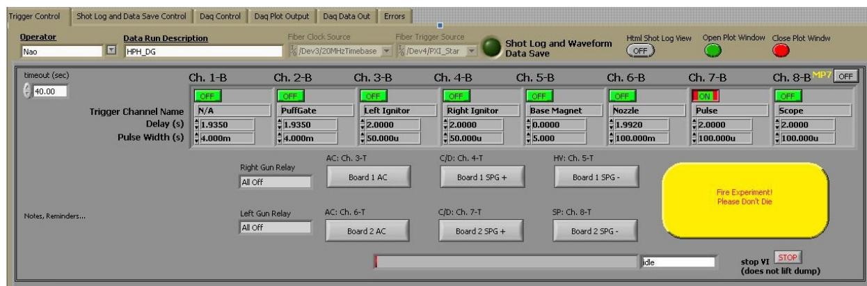
Figure 3.14: Example of parameters set through LabView VI
