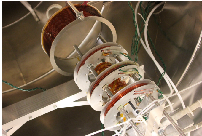
Figure 3.11: Double Gun thruster base field magnetic coils and magnetic nozzle
