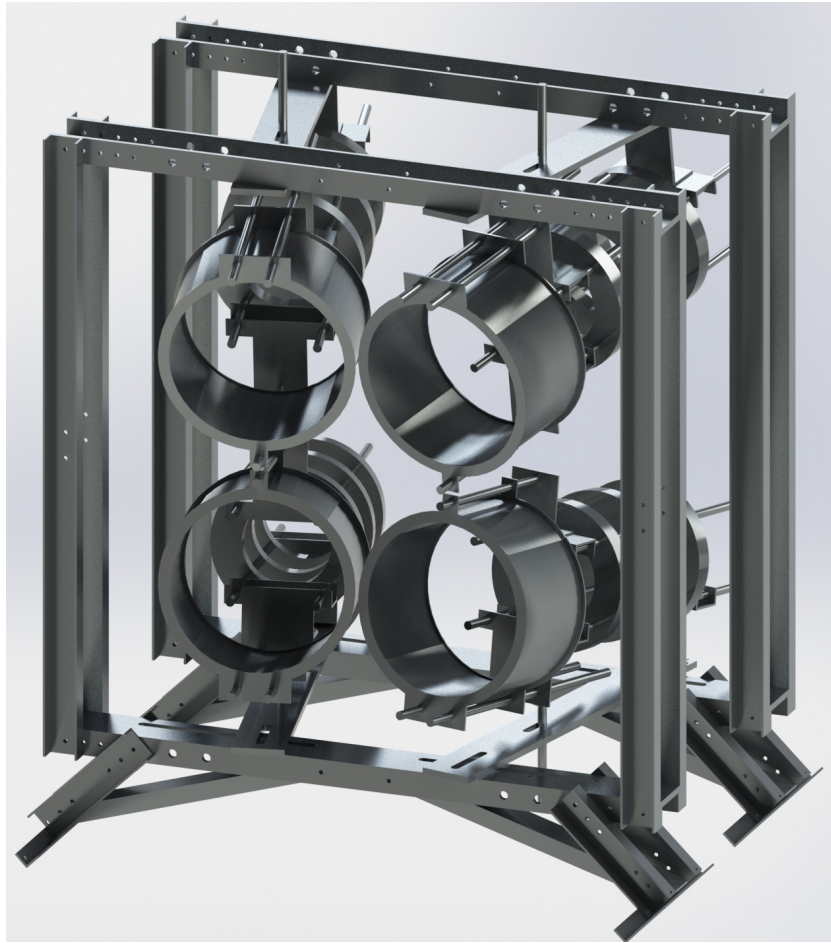
Figure 5.1: CAD rendering of HPH thruster array
