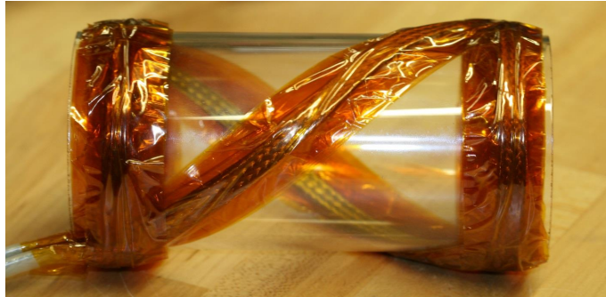
Figure 3.6: Left handed Nagoya Type III helicon antenna
