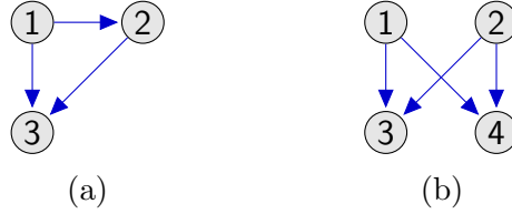
Figure 3.2: In (a), the choice \beta_{31} = \beta_{21} = 1 and \beta_{32} = -1 results in parental unfaithfulness because \pi_{31,\emptyset} = 0 . In (b), the choice \beta_{31} = \beta_{32} = \beta_{42} = 1 , \beta_{41} = 2 , and \mathbb{E}(\varepsilon_1^2) = \mathbb{E}(\varepsilon_2^2) = \mathbb{E}(\varepsilon_3^2) = 1 results in parental unfaithfulness because \pi_{42,3} = 0 .
