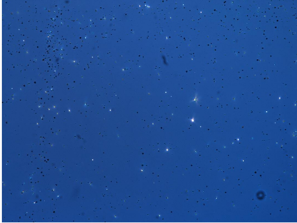
Figure 7: Image from a time-lapse series of calcite nucleation in a 0.3468\text{mm}^2 area with a saturation state of \Omega=7.5 after 72 minutes. Each point represents a nucleus that is growing.
