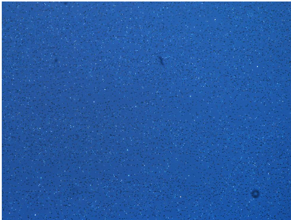
Figure 8: Image from time-lapse series of calcite nucleation in a 0.3468\text{mm}^2 area with a saturation state of \Omega=9.2 after 40 minutes. Each point represents a nucleus that is growing.
