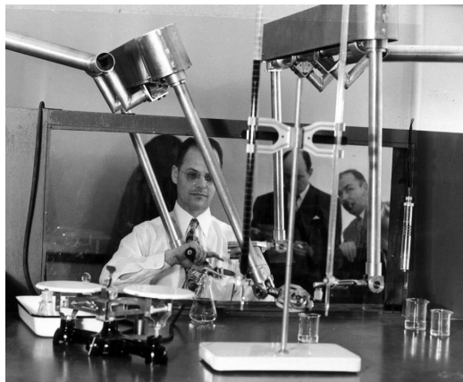
Figure 1.1: Ray Goertz, inventor of telerobotics, safely handles radioactive material using an early mechanical teleoperation system (1951).
