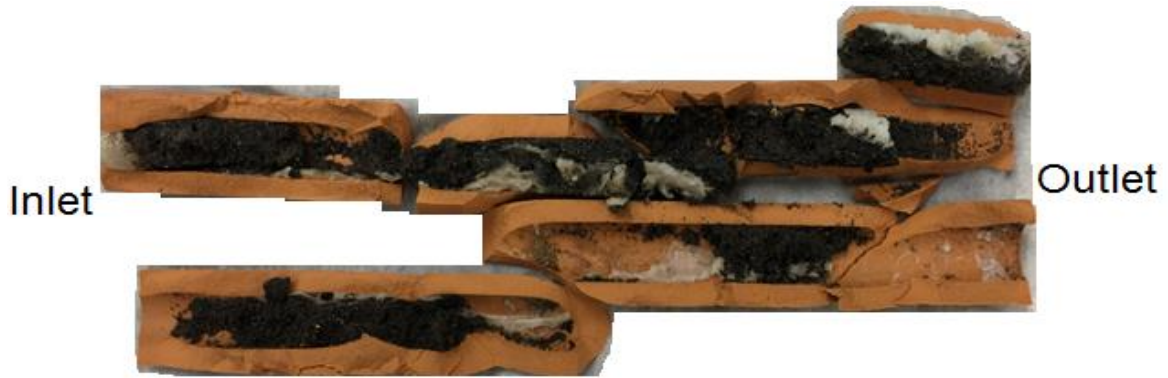
Figure 3.5.2.1 Inside view of the ceramic tube at the end of 3.5 hour injection of 1 mol/L \text{NaHCO}_3 solution in Well 7 groundwater passing through unaffected soil from Well 46 at depth 49-ft: Well 7 groundwater @ flow rate = 1.9 ml/min; 1 mol/L \text{NaHCO}_3 @ flow rate = 0.47 ml/min; Darcy velocity: 2.4 cm/min; Unaffected soil from Well 46C at depth 49-ft
