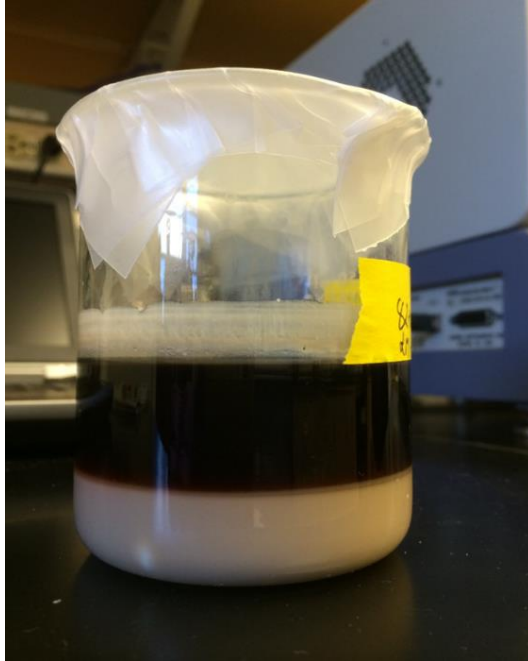
Figure 3.2.1.1.1 Visual appearance of solids precipitated as a result of slow acid addition to groundwater from Well 82 at 100-ft depth (initial pH: 11.786, Final pH: 9.809)
