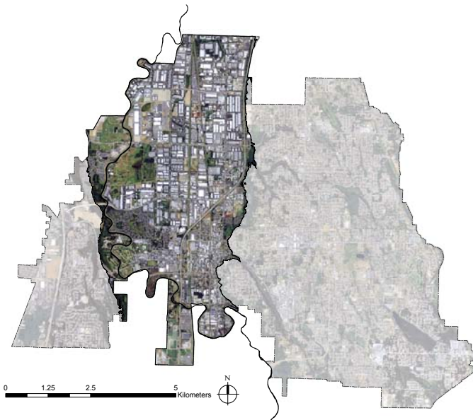
Figure 3-2. The floodplain area within the City of Kent. In this paper a floodplain is defined as the entire area between the valley walls (Anderson et al. 1996). The boundary of Kent’s floodplain is delineated by the 21.3-m (70-foot) contour line. The floodplain has an area of 31.2 km 2 , about 36% of the total area of Kent.
