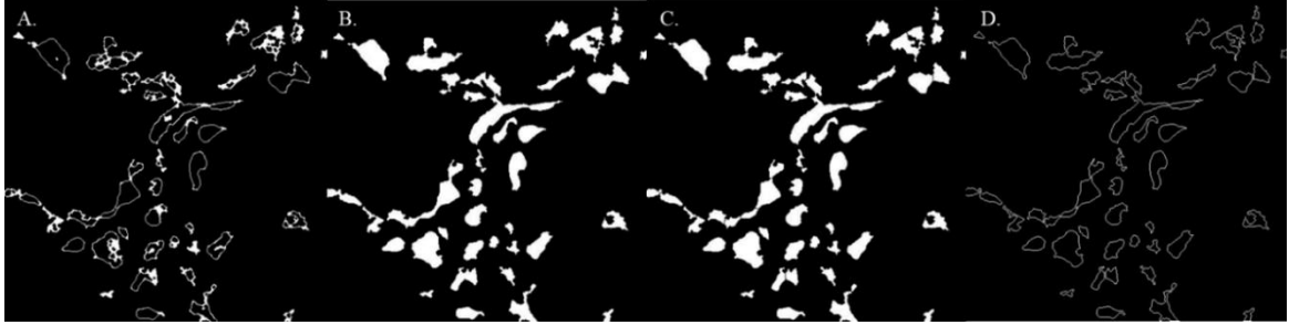
Figure 15: The general workflow for identifying regions of interest in each frame. (A) Borders for each of the regions of interest are generated using an edge-detection algorithm. The cells had borders defined based on neighboring pixels for each pixel of the frame. (B) Cells were filled, and small regions were filtered out. (C) A watershed algorithm was used to aid in cell segmentation. This allowed for the detection of cells that were in contact. (D) Cells were finally converted back into borders for a mask for all the regions of interest. This algorithm was applied for all frames in the recording.
