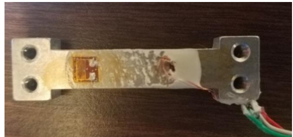
Figure 1: Example of mouse destroying load cell due to not protecting the load cell wiring. A design iteration was performed on the base plate bottom to account for this and to more fully protect the load cell wiring.
