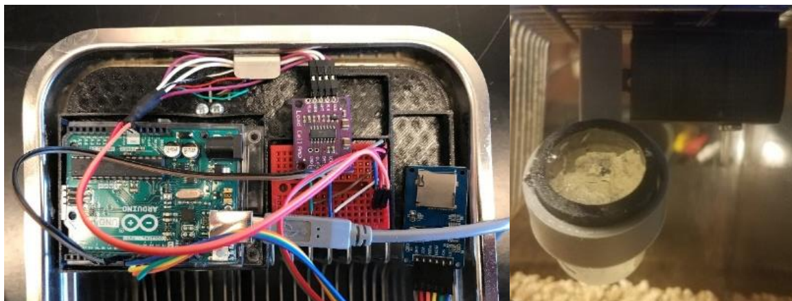
Figure 6: Final setup for the initial prototype of the device. Circuit components consisting of the Arduino, load cell amplifier, and breadboard connected as described (left). Base plate bottom with load cell attached and gel cup holder attached to the load cell, with the gel cup loaded into the gel cup holder (right).
