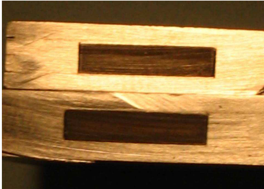
Figure 2.12. Cross section of PZT-NiTi laminated composite.
