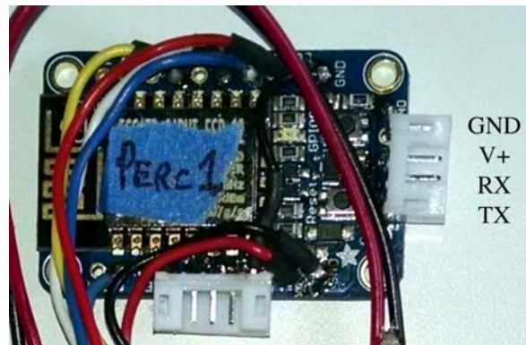
Figure 21: Pinout for the serial port on the Adafruit Huzzah board
