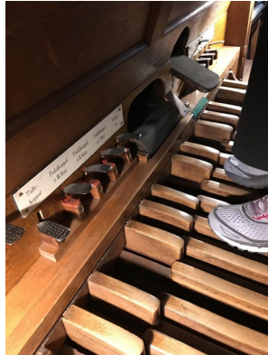
Figure 1.5 Pedalboard of the Wilhelm Sauer organ at Thomaskirche, Leipzig. The cylindrical barrel of the Walze is visible above the center of the pedalboard. 19
