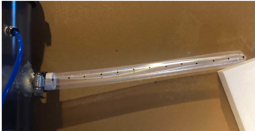
Figure 2.4: An LDPE everted beam deflected a fixed amount
