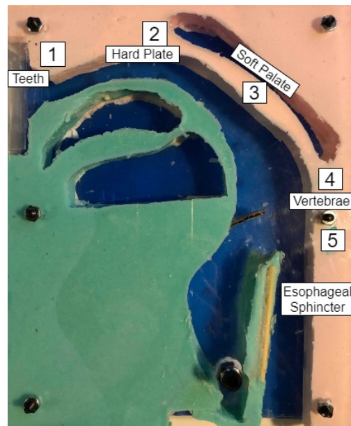
Figure 4.5: Scaled (2X) airway phantom with key anatomical areas highlighted. Hollow pockets in the silicon are included to simulate highly compliant areas of soft palate and tongue. A hinged flap simulates the epiglottis that covers the trachea during eating and drinking.
