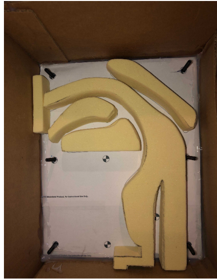
Figure 4.3: Male molds for casting silicone phantom
