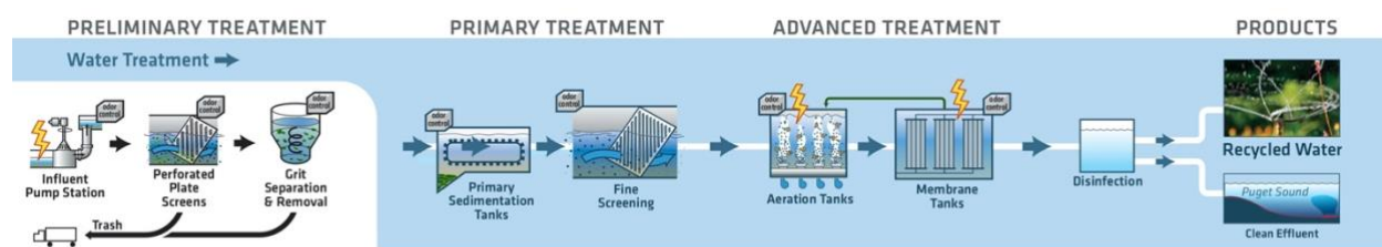
Figure 3-1. Brightwater liquid stream treatment process (King County, 2018) 83 .
