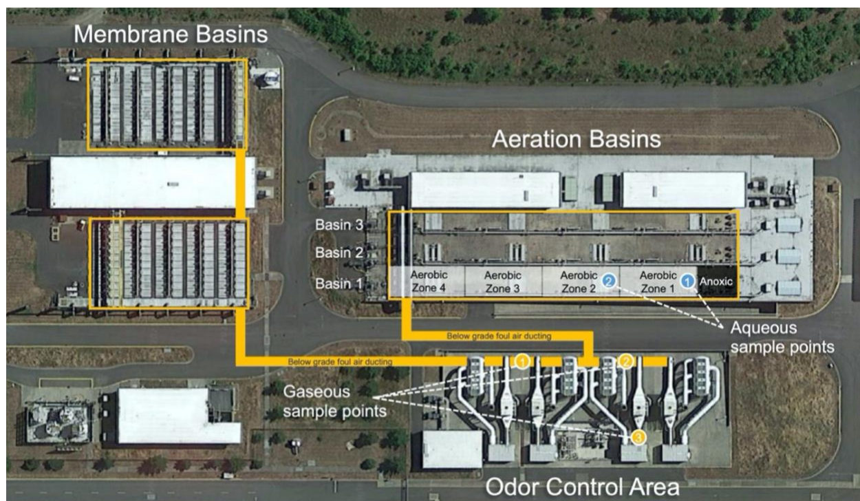
Figure 3-2. Brightwater Treatment Plant with N 2 O monitoring configuration.
