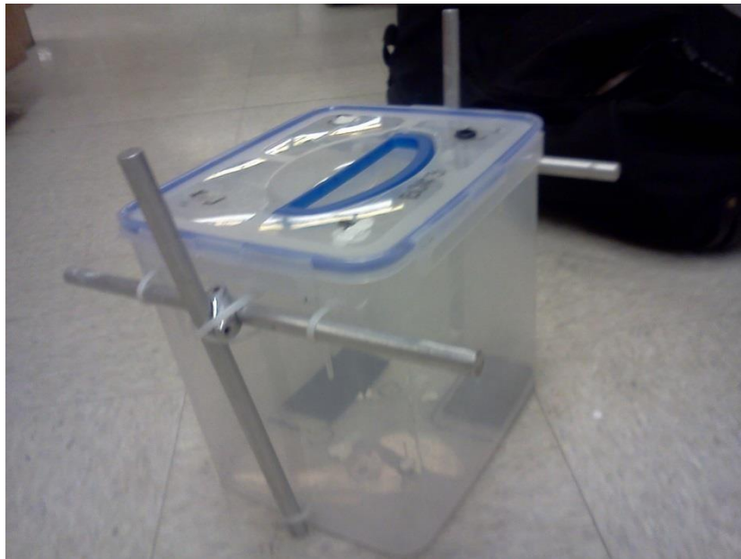
Figure 13: Empty Polycarbonate Case to Contain Sampling Train
